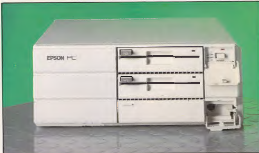
The front panel houses two 5.25in disk drives and the 'Epson PC' badge
